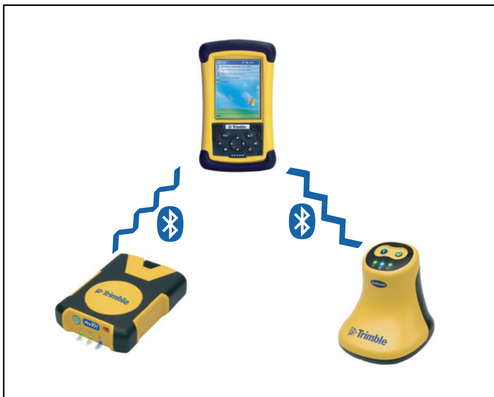
Figure 4 Using a Recon handheld that supports multiple Bluetooth serial ports to connect to a GPS receiver and the GeoBeacon receiver
