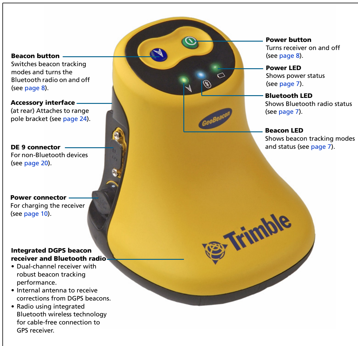
Figure 2 Features and functions of the GeoBeacon receiver
