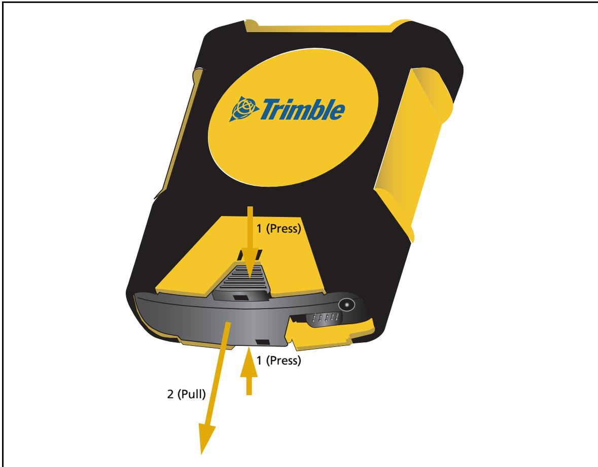
Figure 1.4 Removing the battery
