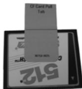
To insert a CF or SDIO card, gently insert the card into the slot. Do not force the card. The pins can be damaged if the card is not aligned correctly.
