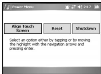
**Align Touch Screen:** A series of targets is displayed. Use a stylus to tap each target to align the touchscreen.
